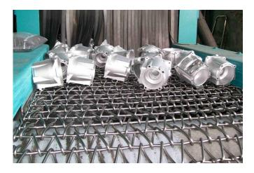
Custom metal belts woven from manganese wire for use in shot blast equipment. Meshes with openings up to 3" are available in wire diameters of .216" or .3125". Most common sizes and specs are available from stock.
