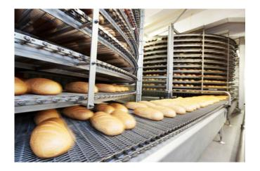
A full line of sprocket driven balanced weave belting is available in carbon and stainless steel for use on transfer and cooling conveyors. Most sprockets are available in SS304 and UHMWPE (ultra-high molecular weight polyethylene) Chain driven belts in carbon and stainless steel for frying and cooking available with custom edges, cleats and attachments for sediment drag out and oil filtering.
