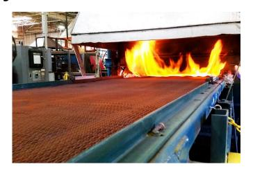
Custom manufactured and designed chain driven belting to increase belt life in your quench and washer belts. Hardening belts available in SS314 & 35/19cb can be manufactured with custom side guards to reduce part
