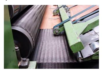
Wire Mesh Belt has been a leader in the manufacture and supply of stainless steel dryer belts for veneer dryers. We can supply dryer belts in any length. Widths up to 240 inches manufactured in Galvanized, 304, 304L, 316ss & 316L with welded, wrapped & welded or looped edges.
